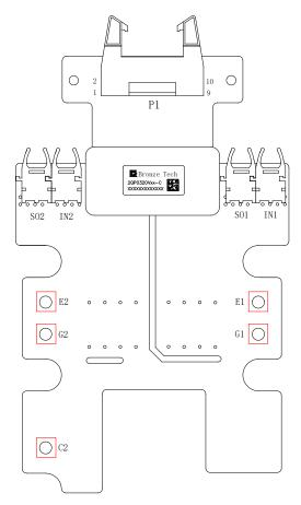
Figure 4. 2QP0320Vxx Pin layout
