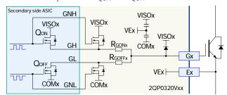
Figure 13. Gate drive output circuitry
