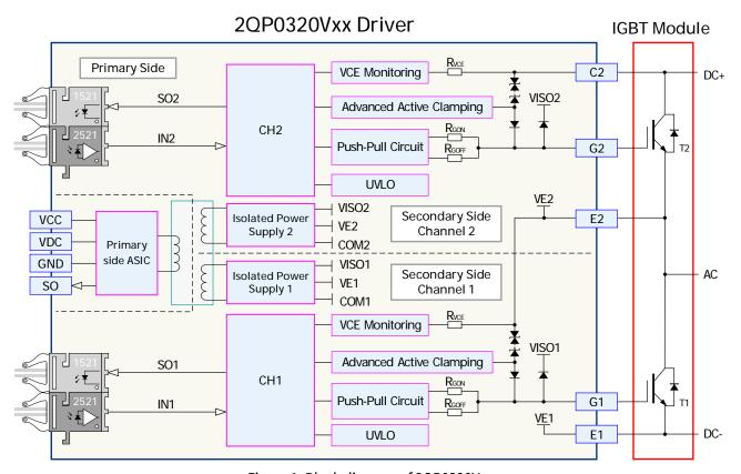
Figure 1. Block diagram of 2QP0320Vxx
