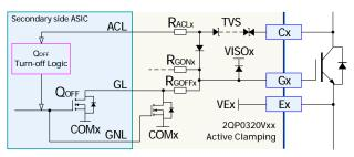
Figure 14. Active clamping circuitry
