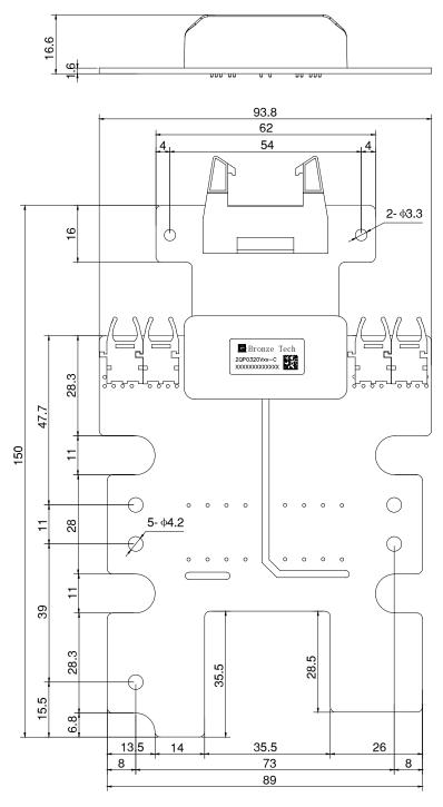
Figure 17. Mechanical drawing of 2QP0320Vxx
