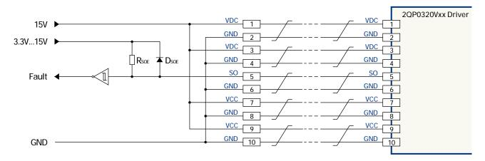
Figure 2. Recommended user interface of 2QP0320VxxA0
