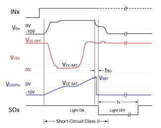
Figure 18. Class II short-circuit protection
