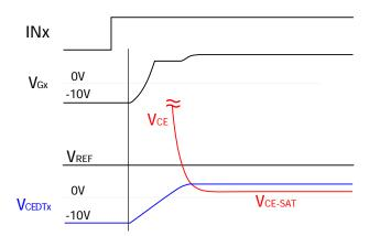
Figure 16. Signal waveform at normal turn-on
