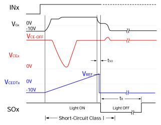
Figure 17. Class I short-circuit protection
