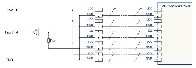
Figure 3. Recommended user interface of 2QP0320VxxC0
