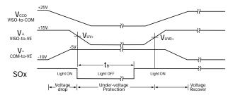
Figure 7. Secondary-side UVLO logic
