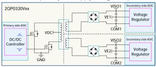
Figure 5. Power supply circuitry
